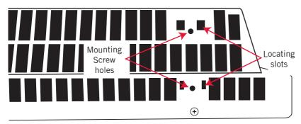
Positioning is only possible in the one orientation, either foot can be used at either end.
